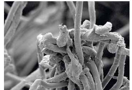
Fracture of a Safety Seat Belt by SEM
