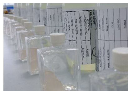
MicrobMonitor jet fuel test
