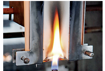
Bunsen burner test set-up
